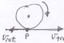
$$V_p = V_{CM} - \omega R = \mu g t - \omega R \quad \therefore V_p = \mu g t - \left( \omega_0 - \frac{2\mu g}{R} t \right) R = \mu g t - \omega_0 R + \frac{2\mu g}{R} t \cdot R = 3\mu g t - \omega_0 R$$
