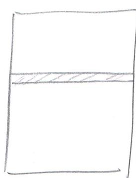
$$\begin{aligned} F_h &= \int_0^h (\rho g x b) dx \Rightarrow \\ &\Rightarrow \rho g b \int_0^h x dx \Rightarrow \rho g b \left[ \frac{x^2}{2} \right]_0^h \Rightarrow \\ &\Rightarrow \boxed{\frac{\rho g b h^2}{2} = F_h} \end{aligned}$$
